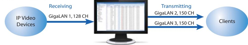
GV-Recording Server + 3 Network Cards assigned on different networks
